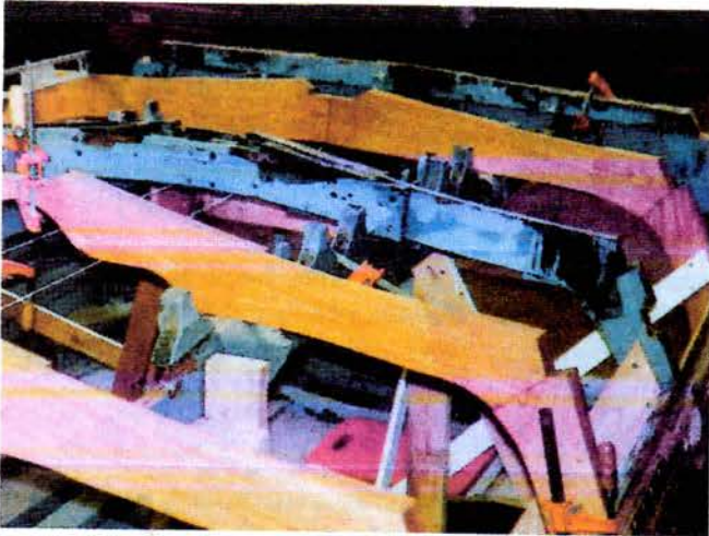
It is a good idea to replace every other frame section using the alternates to verify shape.
