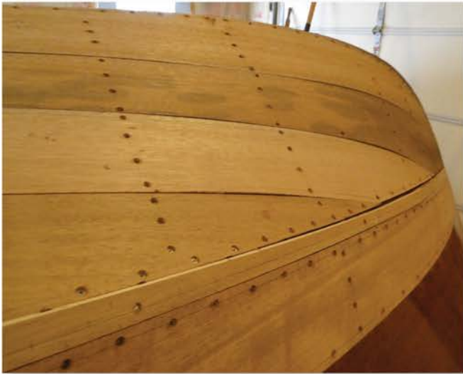
This 'shortcut' 5200 bottom shows almost no rubber filling seams; also stainless screws? Do not expect longevity here.
