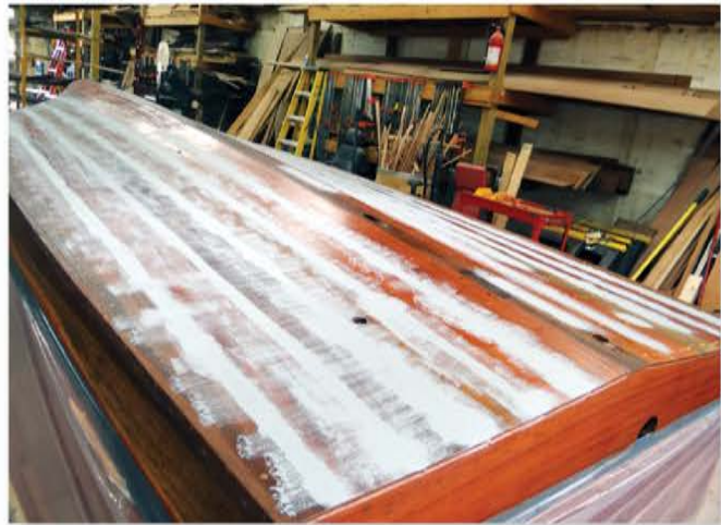
Any remaining tiny gaps, too small to force rubber into, are filled with barrier coat primer by brushing perpendicular to the seams with a stiff brush. Four to five barrier coats follow, then 2 bottom paint.
