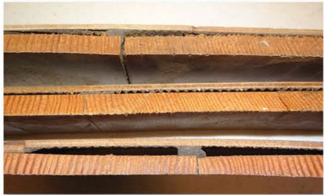
Sections from a failed 3M-4200 bottom. The "professional" restorer used a woefully inadequate amount of 4200 (20 tubes), which set too early (note trowel tooth marks) and he also skipped the use of intermediate frames, which would have pulled the layers together.
