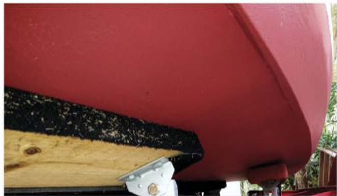
A TRUE 5200 bottom, well used by three owners, 21-years after construction and refresher bottom paint twice.
